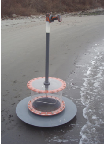
In situ incubation chamber to measure gas flux of restored oyster reefs and suspended oyster aquaculture during EPA-TNC-BU collaborative study. Source: Steven Brown, The Nature Conservancy
