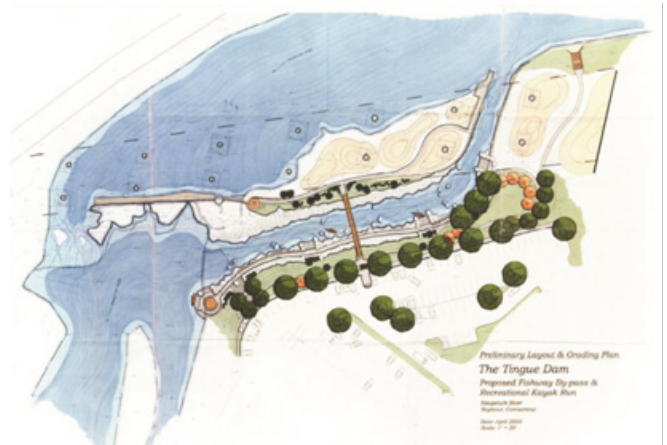
Figure 1. In this architect's rendition of the Tingue Dam Fishway By-pass in Seymour, the Naugatuck River flows from top to bottom, over the dam (gray line to left). As migrating fish approach the dam from below, they will by-pass the dam by swimming up the channel to the right, and re-enter the river further upstream. Source: Milone & Macbroom Engineering, Landscape Architecture, and Environmental Science
