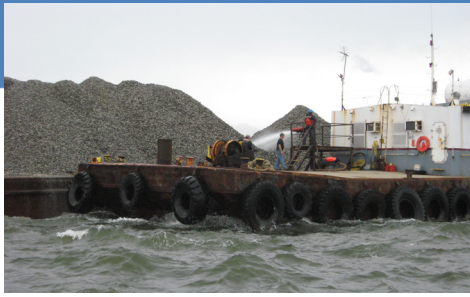
Mined fossil oyster shells are spread on the water bottom in Virginia's James River. Source: Virginia Marine Resources Commission
