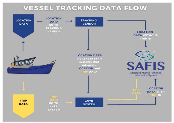
Figure 1. Vessel Tracking Data Flow
